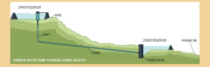
An artist's rendering at top shows the two reservoirs in relation to each other. The pools of water are connected by a penstock, and turbines power a generator. Gravity pulls water down to the lower reservoir when the electrical grid needs energy. At times of low usage, water can be stored above, where the reservoir essentially acts as a battery. Unlike wind and solar energy, which have gaps, the hydro loop can be responsive to demand, whatever the weather.
